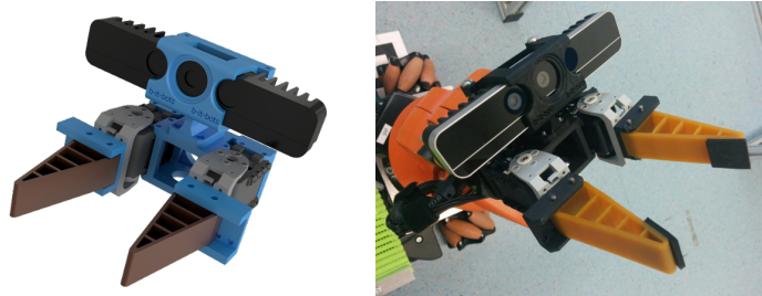
Fig. 2: Custom designed gripper for grasping a wider range of objects.
